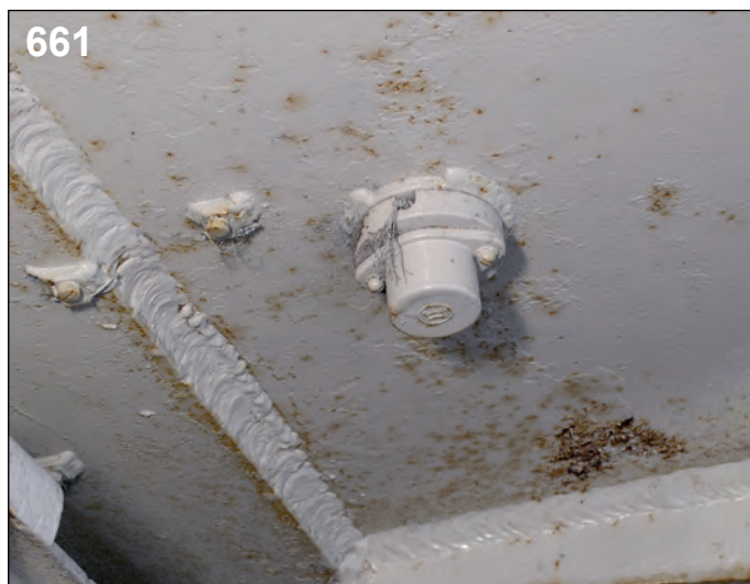
661: The graticules at the forward end of the gun sight could be illuminated by a plug-in lamp unit. This lamp unit was also fitted with a dimmer switch and was powered by a plug from the 12V socket attached to the turret roof above the gun sight mount.
