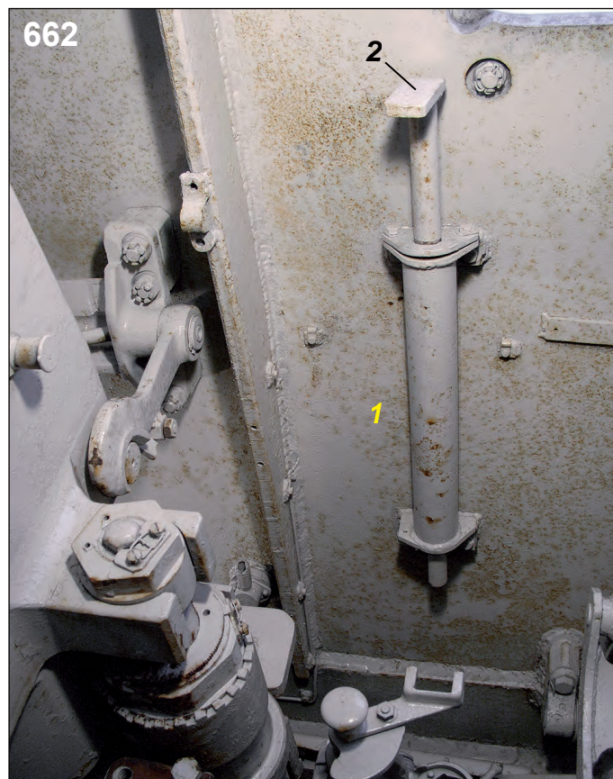
662: Of primary interest in this photo is the large spring balance cylinder seen at 1 . When the loader closed his hatch the arm at 2 , page 161 , illustration 667 , contacted the end plate, at 2 , thus allowing the damper spring to slow the closing of the hatch.
