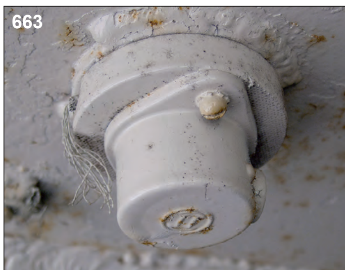
663: A view of the Bosch 12V socket seen in photo 661 . This was named, Steckdose für Strichplattenbeleuchtung , and two of these were fixed to the turret roof. These sockets powered the gun sight graticule light and the main gun firing circuit
