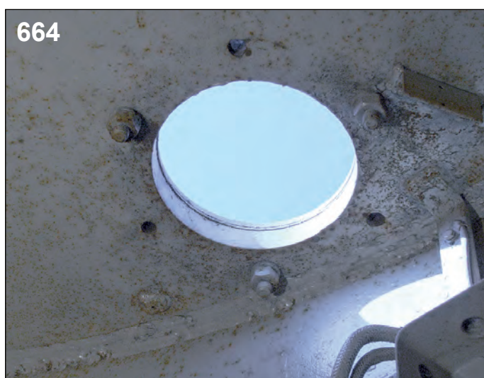
664: Fitted into the turret roof was an extractor fan that was used to exhaust fumes from the turret after firings of the main gun. This fan, the Aufbaulüfter , had an airflow extraction of 12 3 /min.
